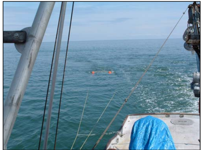
Surface trawling for juvenile salmonids with modified 3.0 m by 3.0 m Kvichak trawl
