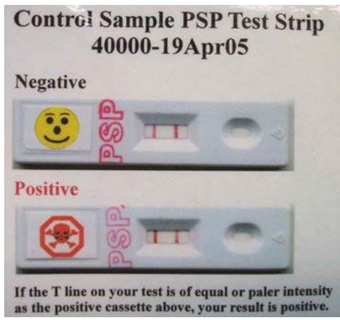
Figure 2. Jellett test strip line interpretation card used to determine if test results are positive or negative.
