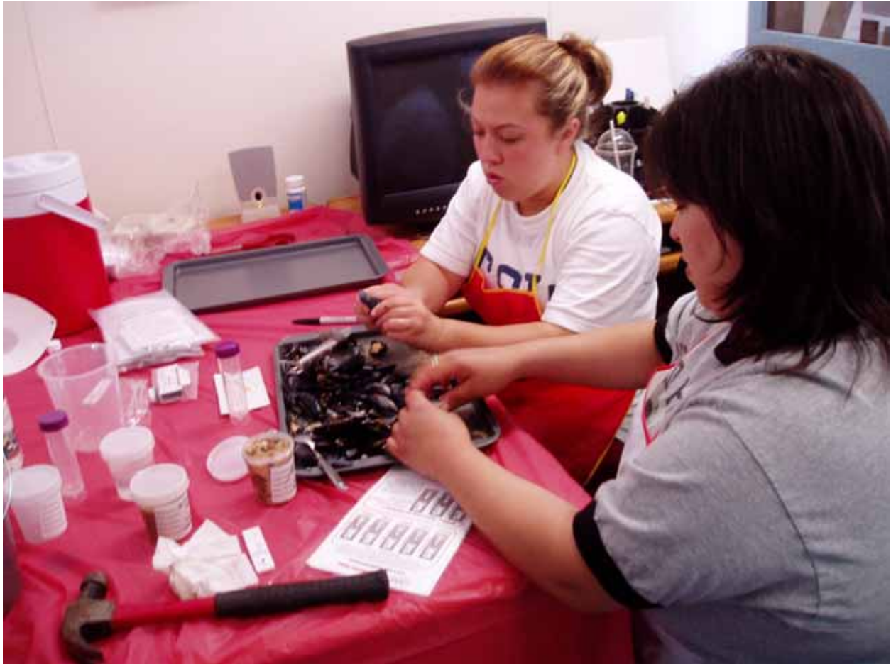
Sand Point technician, Dana Osterback (left), and her assistant prepare a sample of mussels to be tested for PSP. About 40 medium mussels were needed for the test. Photo by Bruce Wright.
