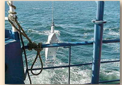
CPR 161 suspended from the davit prior to streaming in the sea at 15 knots. (Sonia Batten)
