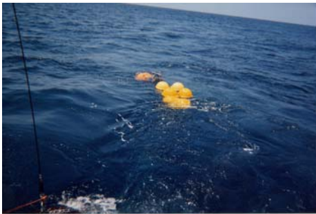
Recovering a mooring. The large orange instrument contains an ADCP which measures currents. The yellow balls keep it upright.
